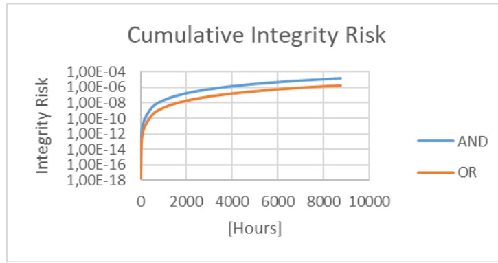
Figure 2: Integrity Cumulative Risk for a Fully Dual-Redundant Architecture
