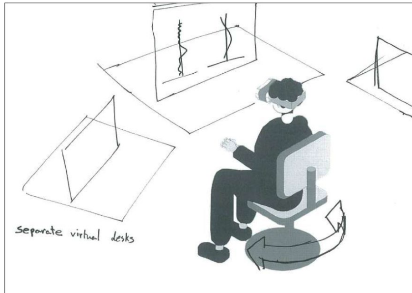
Figure 7. With this setup, the glasses will project multiple different screens for the operator to choose from. Here the operator is able to setup the screens to view the desired information.
